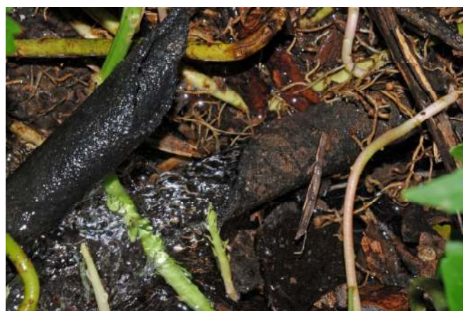
Damaged Soaker (Drip) Hose Gushing Water
