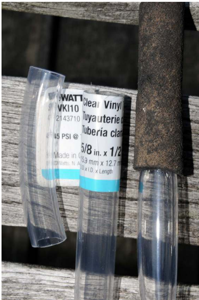
Center: Clear vinyl tubing, 5/8 inch outer diameter. Left: Short, about 2 inch length of tubing for insertion. Right: Short length of tubing inserted into soaker hose.
